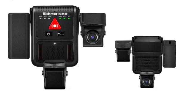
BK6 Mini size (just bigger than a Camera), portable with cheap transportation. Powerful function, High integration. Support3G/4G, GPS,WIFI, G-Sensor, Talkback, TTS...function. Easy installation.
