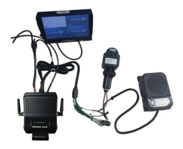
PIR is a device that recognizes screen changes. When PIR detects a screen change, it will generate a high level to the device to generate an IO alarm. When our device detects the IO signal, it will link with the platform to generate several functions | Sleep wake-up, attachment upload, email push
