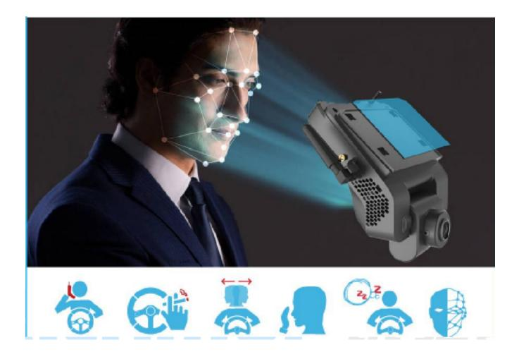
DSM driver status monitoring/fatigue detect
