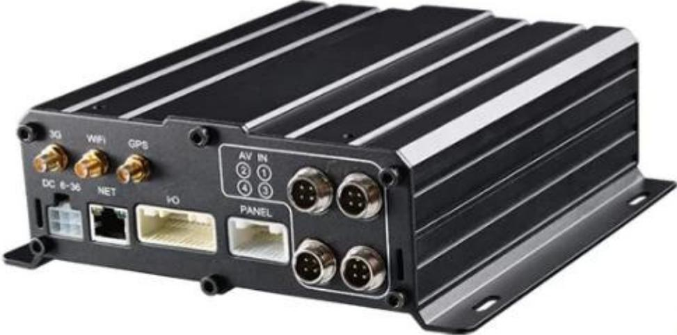
The image shows a black, rectangular mobile DVR device with a ribbed top surface. The front panel features several ports: a 3G antenna, a WiFi antenna, and a GPS antenna; a DC 6-36V power input; a NET (Ethernet) port; an IO (USB) port; and a PANEL port. There are also four circular connectors labeled AV IN (1, 2, 3, 4). The device is shown from a three-quarter perspective.
